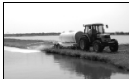
Figure 6. Hydrated lime slurry being applied with a pull-behind sprayer.
