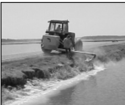
Figure 5. Hydrated lime being applied to a pond with a tractor-mounted auger.
